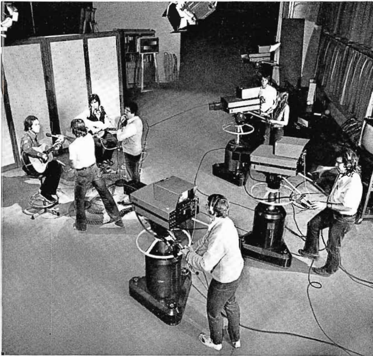
Studio D at WHA-TV is used by the University Department of Communication Arts for teaching television production. Four TK-630 cameras in this 40' x 50' studio provide ample opportunity for students to obtain "hands-on" operating experience.
