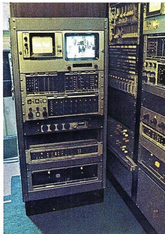
One of Opryland Productions' seven TK-45 cameras has a custom, rack-mounted CCU complete with test facilities, sync generator, and audio mixer. This rolling rack permits using the camera with the mobile unit or at the studio.
