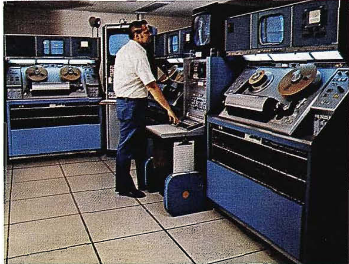
Camera control area is spacious and uncluttered. Engineer Don Bednarek rides video on one of the six TK-44B cameras operated from this position. Console also includes controls for 1—TK-28 Film System; 1—TK-27 Film System, as well as Pulse assignment and Genlock. Intercom system is a BCS-5000.
